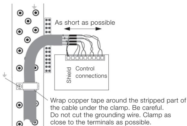
**Figure 3-10 Essential points for control cabling transit.**
