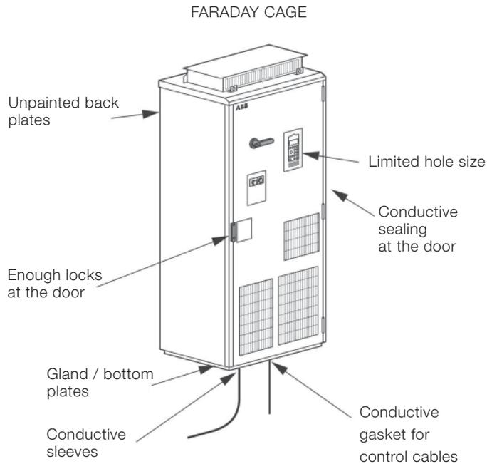
**Figure 3-4 Typical enclosure aperture detail.**
