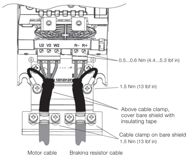
**Figure 3-8 360° earthing with clamping of cable shield.**
