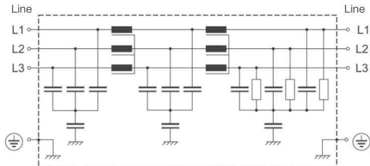
**Figure 3-3 Example of filtering integrated in drive module.**
