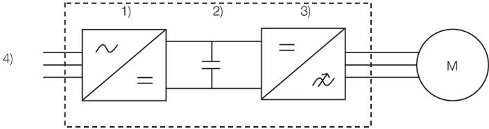
Figure 2.1 A single frequency converter consists of 1) rectifier, 2) DC-link, 3) inverter unit and 4) electric supply.
