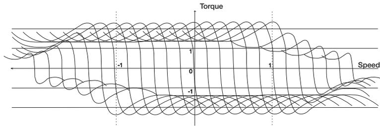
**Figure 4.2** Torque/speed curves of an induction motor fed by a frequency converter.  $T_{max}$  is available for short term overloads below the field weakening point. Frequency converters, however, typically limit the maximum available torque to 70% of  $T_{max}$ .
